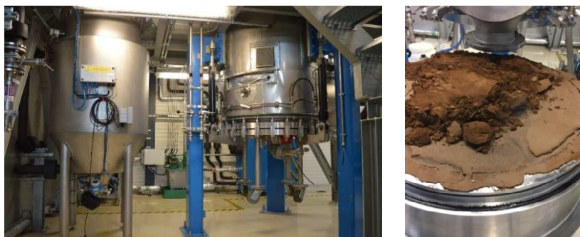
Figure 13: Precipitation tanks and crystals obtained after FDCA recovery by precipitation at pilot scale
